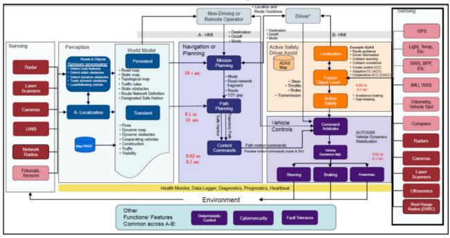
Figure 10.1: SAE International Autonomous Mode Functional Architecture Flow Diagram
