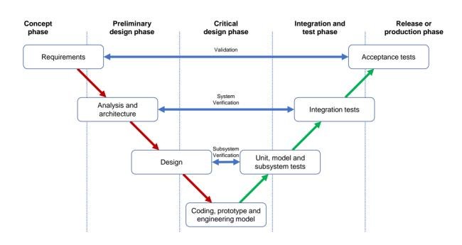
Figure 9.1. Engineering 'V' diagram showing system development lifecycle
