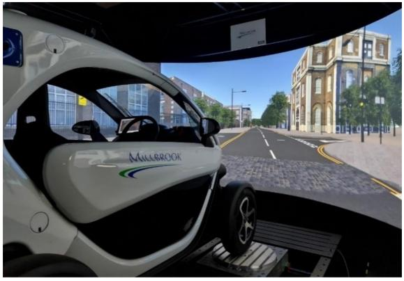
Figure 5.16: Millbrook vehicle simulator (Vehicle in the Loop Simulation)
