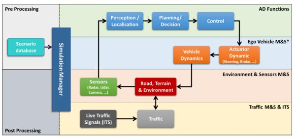
Figure 4.3: Interoperable Simulation Environment as System of Systems
