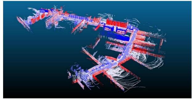
Figure 5.10 Route A Point cloud map generated from virtual Lidar sensor (Claytex) in rFpro
