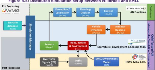
Figure 4.5: Distibuted Simulation setup between Millbrook and SMLL
